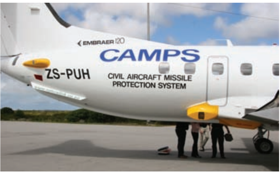
The photographs on these two pages show the positioning of the system's yellow-painted sensors and dispensers on the nose and rear fuselage of the Embraer 120 aircraft
